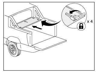
Push both left latches away from you to lock the latches (remember that there are two latches on each side for panel 1). You should hear a click when each latch locks correctly. Lock the remaining two right latches on panel 1.
